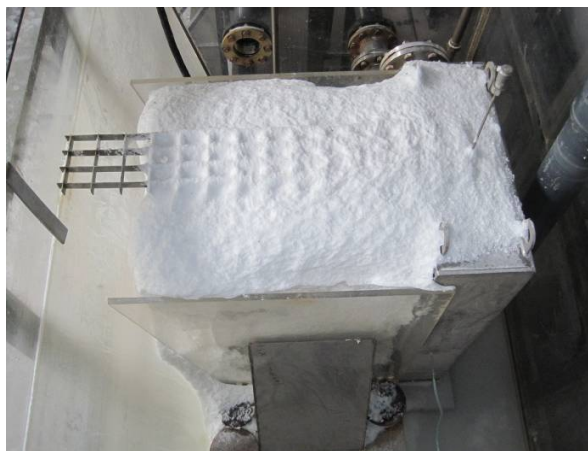
Fig. 17. Post-test photograph of full fiber/particulate load test
